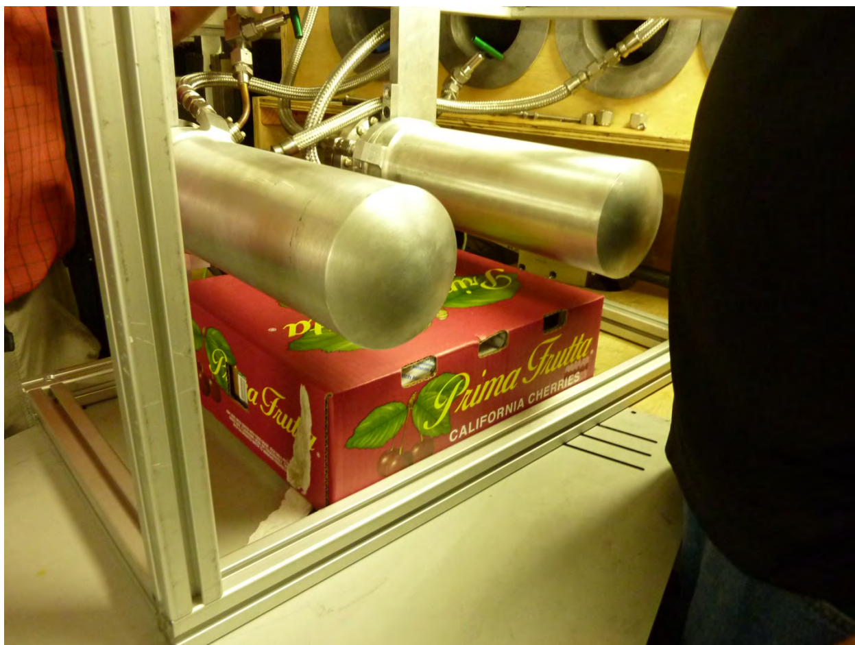
Fig. 1. Experimental set-up using 4-Pi X-ray tubes to irradiate boxes of sweet cherries.
